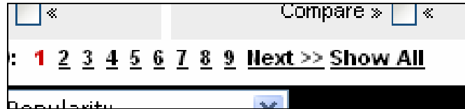
Figure 4.3 A "Show All" link embedded after a series of sequential links. Note that this link has the same style of the surrounding links, so it appears like a natural part of the page. Clicking this link will cause the browser to start downloading the other links shown here and concatenating their content to the current web page.
